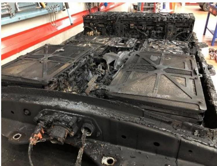
*Fig. 3. - Battery disassembly process after the test.*
