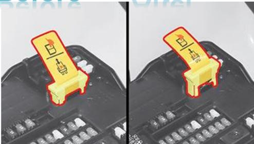
\*The yellow lever doesn't get pulled out completely.
