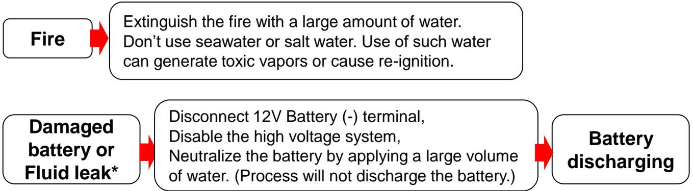
\*To be used if electrolyte solution leakage or damage to the high voltage battery casing is observed. Check battery pack temperature with thermal imaging camera.
