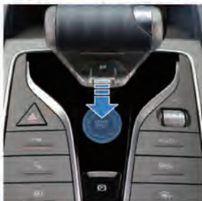
Turning off (Power meter "OFF")
