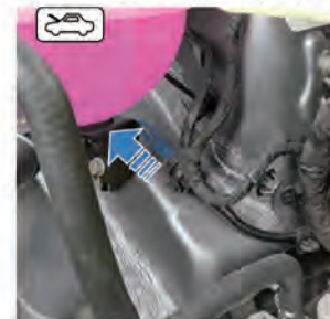
Disconnecting from the charging station (emergency release)
