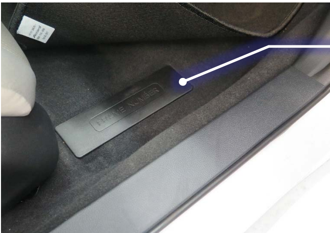
Stamped into the floor panel in front of the passenger seat under a plastic panel marked FRAME NUMBER
