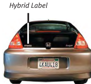
Depending on the model year, a hybrid label will appear on the right or left rear of the vehicle.
