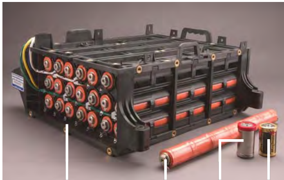
HV Battery Module Single HV Battery "Stick" Single HV Cell D-Cell Battery
