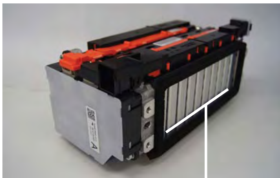
One of Four Battery "Stacks"
