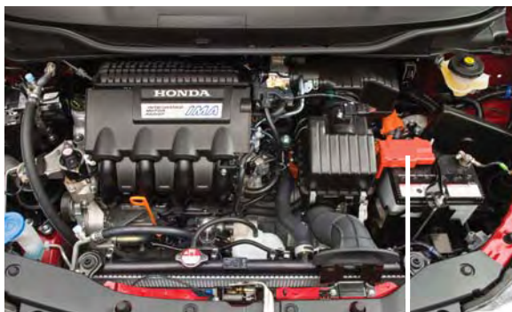
Positive Battery Terminal
