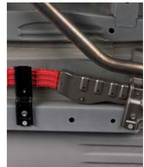
Thermal shield near hot exhaust
