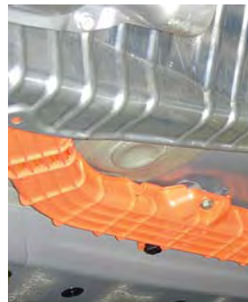
Electrical shield bolted to undercarriage
