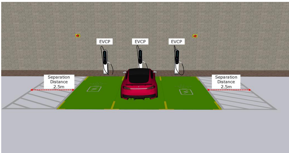
Figure 5: EVCB with AC Charger Located Outdoor in New Development should be Separated by a Distance of 2.5m from Non-EV Parking Bay
