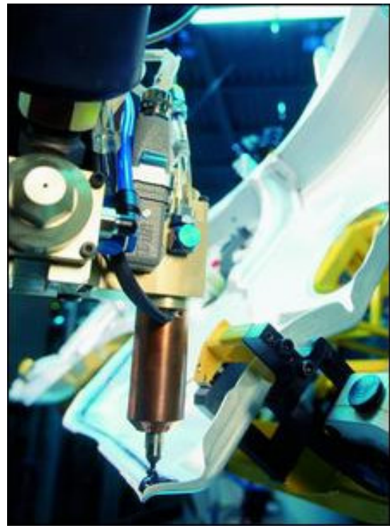
Riveted casting for front strut tower on new Jaguar XK sports car
