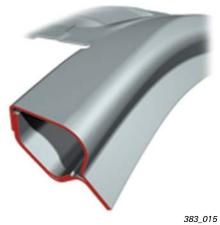
A-post, Audi TT Sheet-aluminium sections (interior/exterior)
