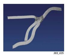
Micrograph of the roof frame and roof panel joint
