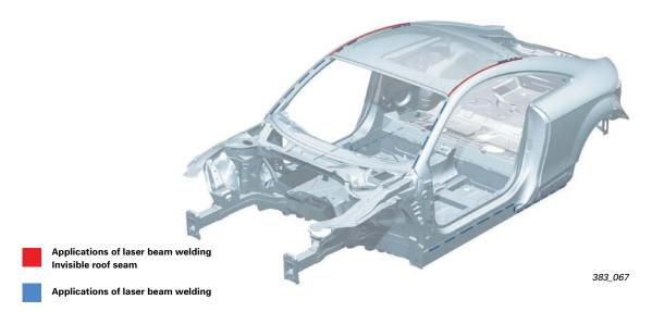
To ensure consistent laser welding of aluminium parts, the parts to be welded must have a perfectly clean surface. This is achieved either by washing the component parts followed by chemical pickling or by using the new Laser Clean process.
