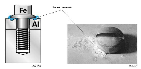
Schematic of contact corrosion with example
