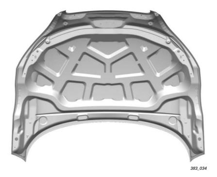
The overall concept provides for deformation zones between the bonnet and the units or car body structural parts.
