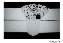
Micrograph of a laser-welded seam with Laser Clean (above) and without cleaning (below)
