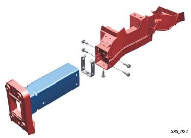
Joint between beam 1 and beam 2
