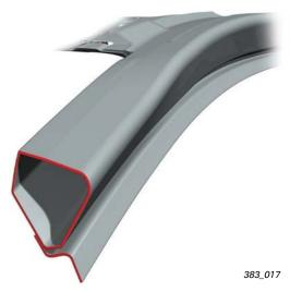
A-post, Audi A8 Single-chamber extruded section
