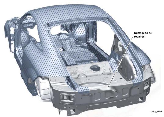
body parts which must be covered when carrying out steel repairs
