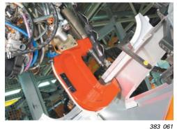
Solid punch riveting process in production
