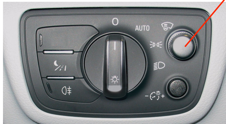
Position controller for head-up display, Windshield Projection Head Up Display Button E736
