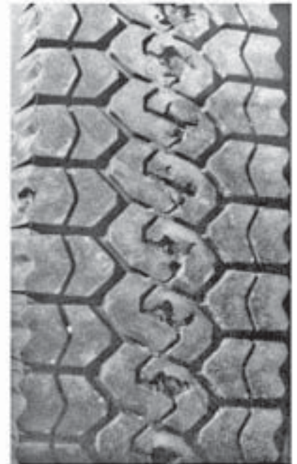
Example of Dyno Damage
